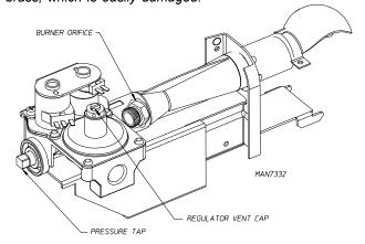
Reinstall the burner tube onto the burner base.
