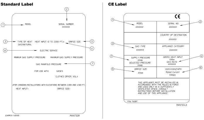
When contacting Maytag, the information on the data label is required to ensure proper service/parts assistance. The data label is located at the upper left rear of the dryer behind the back guard.
