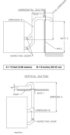
**NOTE 1** Opening from combustible materials must be 2-inches (5.08 cm) larger than the duct (all the way around). The duct must be centered within this opening.
